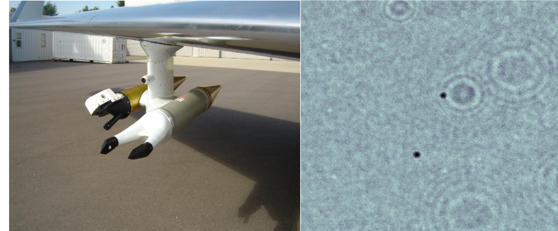
Fig. 1 (left) HOLODEC attached below the aircraft wing (source: NCAR), (right) hologram with detected droplets.
