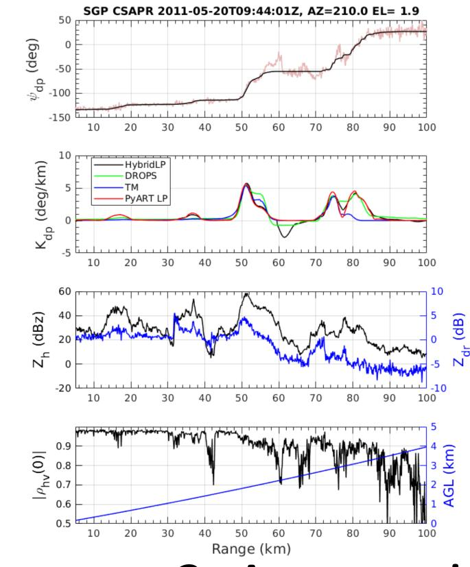
Additional global constraints on total delta  $\Phi_{DP}$  provides a weighting between local and global scope effects. Works in situations with backscatter differential phase effects. Gives estimates with and without positivity
