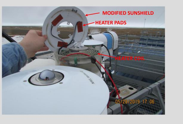
8-48 5/28/19: Heater coil, heater pad on bottom of sun shield, modified sun shield opening.
