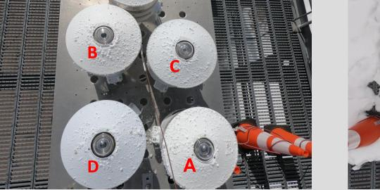
5/9/19, 2:14 MST: "C" modified sun shield first to clear dew in cooling cap test on PSP dome.
