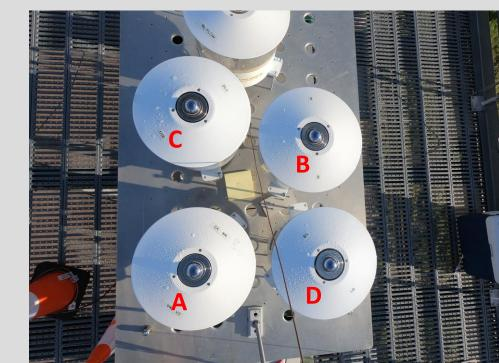
5/12/19 17:45 MST: "B" and "C" modified sun shields averaged quickest PIR dome drying in water spray tests.
