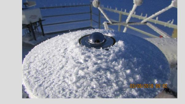
PIR1 3/8/18: Modified sun shield with widened opening. No frost on dome. Frost and snow on sun shield.
