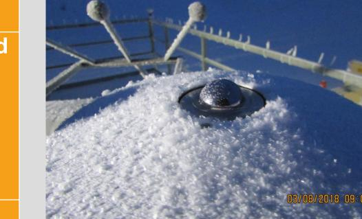
PIR2 3/8/18: Standard sun shield. Frost on dome. Frost and snow on sun shield.
