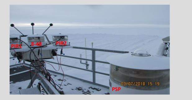
PSP 3/7/18: Heater pad installation significantly reduces frost, snow on PSP dome and sun shield. Snow is on top of PIR and 8-48 sun shields.
