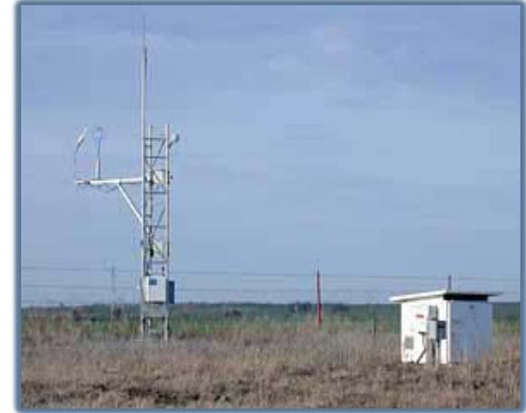
Water vapor fluxes, latent and sensible heat, carbon dioxide
