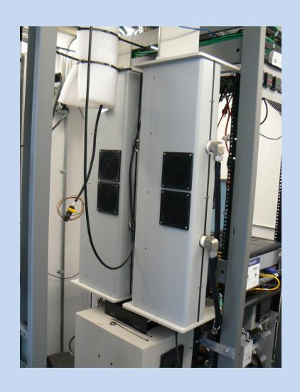
The f(rh) consists of two components two nephelometers, ambient and sample and an aerosol humidifier
