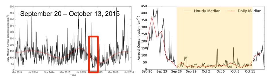
Daily <u>accumulation mode</u> (~ 100 nm – 1  $\mu$ m) < 50 cm<sup>-3</sup> for ~ 2 weeks Can we see evidence for aerosol removal by precipitation? What allowed very low CCN conditions to persist for 15 days?
