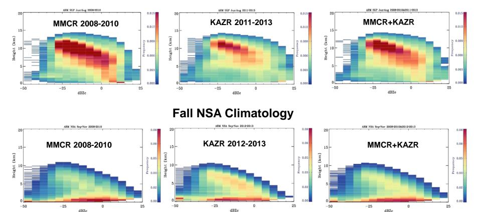
MMCR show much higher frequency of occurrence in middle and upper levels at SGP and near surface at Barrow
