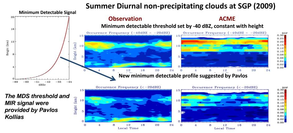
• The overestimation of high non-precipitating clouds in ACME is largely due to the limitation of Radar to detect weak signals
