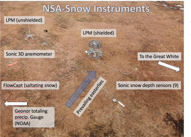
Extensive sets of instruments have been installed at Barrow and Oliktok to characterize frozen precipitation. The mentors Jennifer Delamere and Matthew Sturm are actively working with these instruments.
