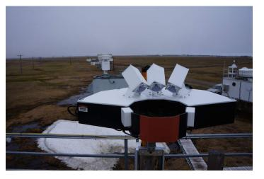
The multi-angle snow camera (MASC) provides highresolution images of ice particles, fall speeds, and particle morphology at Barrow.
