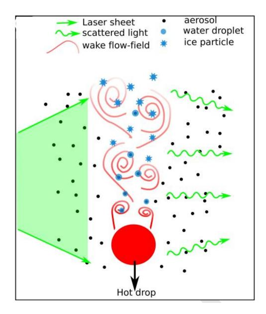
Observe droplet activation or ice nucleation in the wake of large, warm falling drops.
