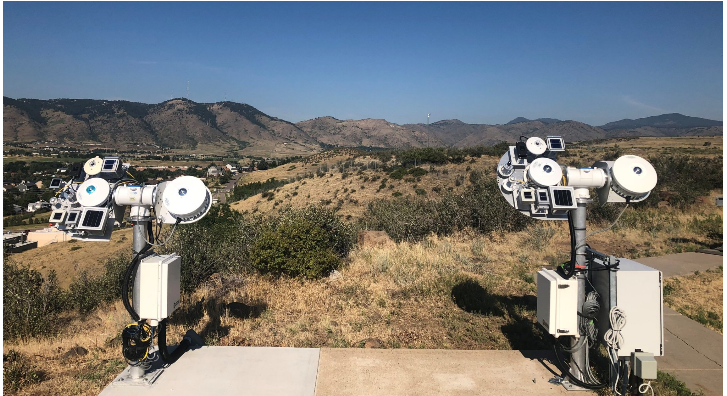
2 and 1-axis tracking WISER – Installed Jan 2020 & Oct 2017
