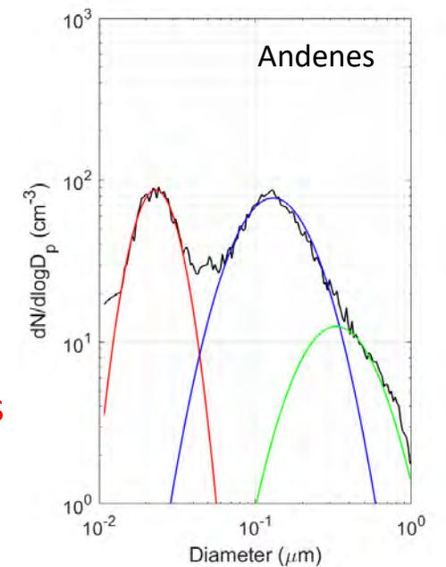
Fig 1: UHSAS and SMPS measured size distribution (black) with modal fits (red, blue, green) for 3/13
