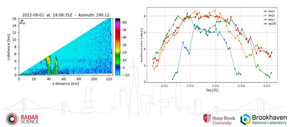
Multi-Doppler wind retrievals are performed for each CHIVO gridded (composed of 4 RHIs) using nearest gridded CSAPR2 and NEXRAD The multi-Dop outputs every ~40 sec.
